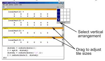
You can control the relative positions of the command window and the worker output. The following figure shows how to set the output to display beside the input, rather than above it.
