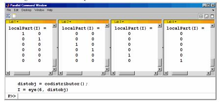
Alternatively, if the data is distributed by rows, you might want to stack the worker tiles vertically. For the following figure, the data is reformatted with the command
