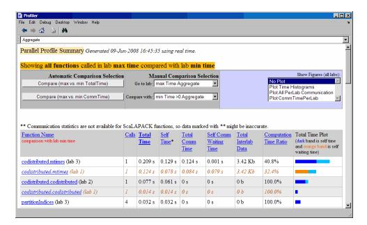
Select a function name in the summary listing of a comparison to get a detailed comparison. The detailed comparison for codistributed.mtimes looks like this, displaying line-by-line data from both workers:
