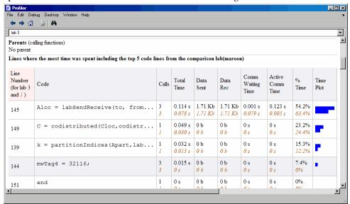
The following figure shows a summary of all the functions executed during the profile collection time. The **Manual Comparison Selection** of **max Time Aggregate** means that data is considered from all the workers for all functions to determine which worker spent the maximum time on each function. Next to each function's name is the worker that took the longest time to execute that function. The other columns list the data from that worker.
