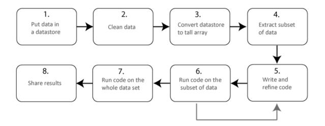
The illustration shows a typical workflow that uses tall arrays to analyze a large data set. In this workflow, you analyze a small subset of the data before scaling up to analyze the entire data set. Parallel computing can help you scale up from steps six to seven. That is, after checking that your code works on the small data set, run it on the whole data set. You can use MATLAB to enhance this workflow.
